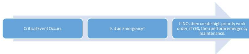
Fig 13.2: Work Flow of Emergency Maintenance
